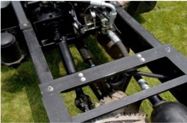
**Close-up of the driveline used for the parallel hydraulic hybrid** - *Colorado State University*
