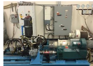
Hydraulic Hybrid Transmission HIL Test Rig with Electric Engine and Vehicle Emulators
